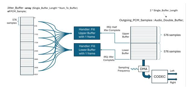
Each UDP packet contains 576 PCM samples, used as the *single buffer length* for the double-buffered Outgoing PCM Samples and the Jitter Buffer.
